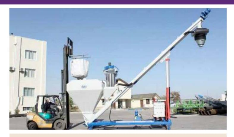
Material, discharged from the blade-cut Flexible Intermediate Bulk Container (FIBC), undergoes a controlled transfer helped by the screw feeder. The material is seamlessly conveyed to the telescopic loading bellow, ensuring a dust-free environment during the loading process into the tanker.
