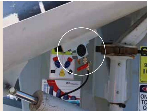
OT (Turbine vibrator) - Chute on concrete mixer
